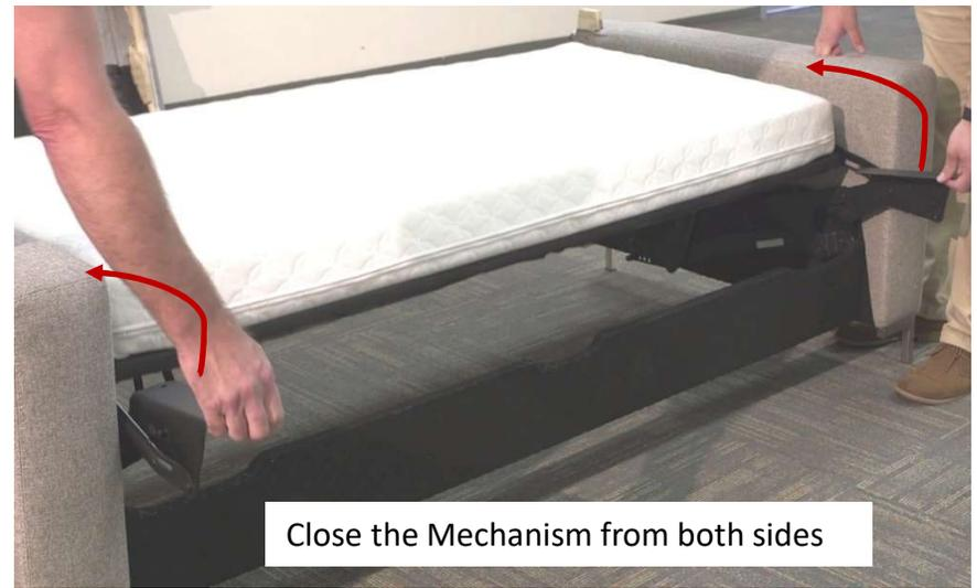
Close the Mechanism from both sides
