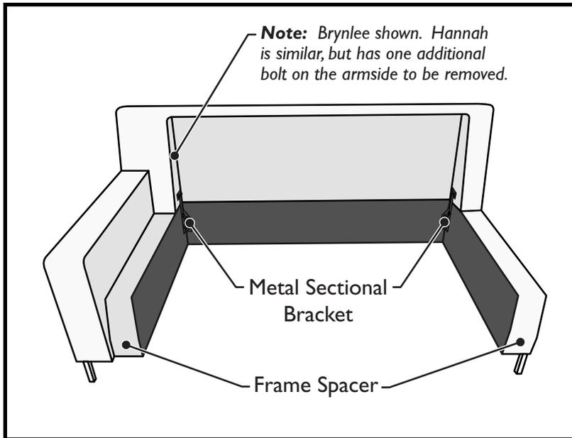
**Figure A.** Sectional Brynlee (BRY) and Hannah (HNH) comfort sleepers have a *frame spacer* on each side, as well as a *metal sectional bracket* on each side. The *metal sectional bracket* secures the back to the *frame spacers*.
