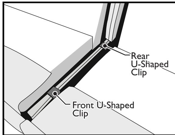
3. Install the second U-shaped clip towards the back of the armless side panels as shown in the picture above. With both U-shaped clips in place, the sectionals will be secure.
