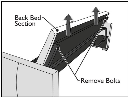
6. Remove (4) four bolts on each side of the comfort sleeper that secure the back bed section to the mechanism. Start from the bottom, leaving a single top bolt on each side. Hold the back bed section while removing the last two bolts. Set the back bed section aside.
