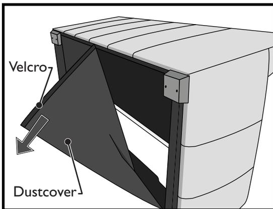
3. Roll the comfort sleeper forward, as shown. Open the dustcover on the bottom by pulling to release the velcro holding it closed.
