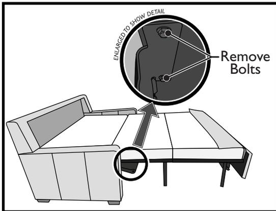
1. To begin, open the comfort sleeper as shown. Remove the two bolts connecting the middle bed section to the mechanism, as shown in the enlarged view. Do this on both the left and right sides.
