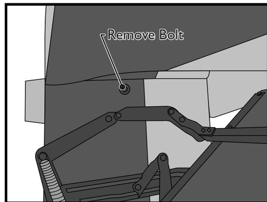
4. With the dustcover open, you have access to the bolt securing the arm to the back. Remove the bolt, as shown in the figure above, from both sides of the comfort sleeper.
