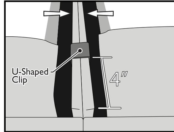
2. Use one hand to squeeze the armless side panels together. Use the other hand to slide the U-shaped clip over both decks as shown. Place the U-shaped clip about four inches from the front of the armless panels as shown in the image above.
